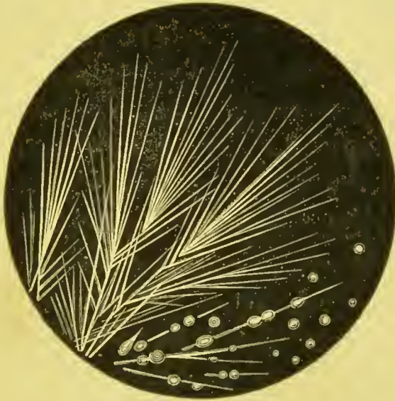
FIG. I.—Glycocholate of soda from ox-bile after two days' crystallisation. At the lower part of the figure the crystals are melting into drops from the evaporation of the ether and absorption of moisture. After J. C. Dalton.
